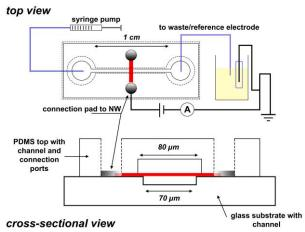
Figure 2: Top and cross-sectional schematic of the glass-PDMS device. The NW is depicted as a red stripe. Electrical contact is established with the NW through ports punched in the PDMS.
